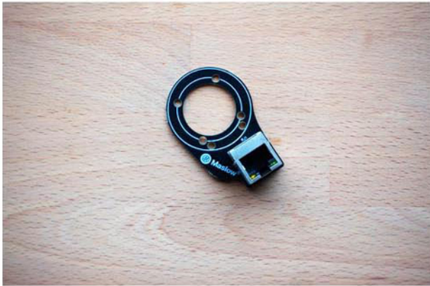
Magnetic Encoder Board. Quantity 4 Properties: AS5600 magnetic encoder with ethernet interface.
