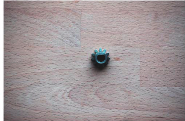
Drive Gear. Quantity 4. Properties: Steel, Fits D-shaped 8mm shaft with set screw.
